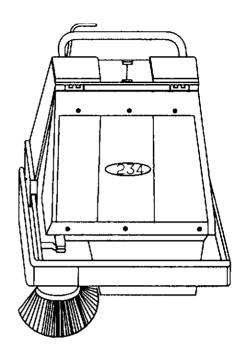
Figure 3-3 Battery-Powered, Walk-Behind, Mechanized Sweeper
