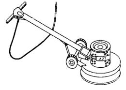
Figure 3-1 Low RPM Floor Machine 160 to 185 RPM
