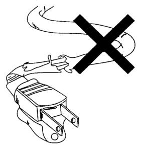
Figure 2-3 Frayed Cord, Ground Prong Missing
