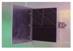
Remove and replace primary filter as needed.
