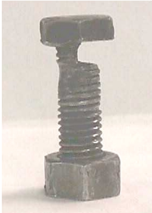
Figure 3. Worn Non-SAE Grade 8 Bolt
