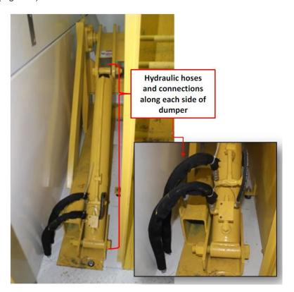
FIGURE 6. Check Hydraulic Hoses
