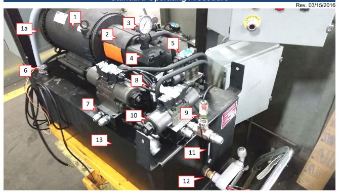
Figure 31. Hydraulic Power Unit—Major Components
