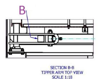
Figure 23. Top View of Dumper Cylinder
