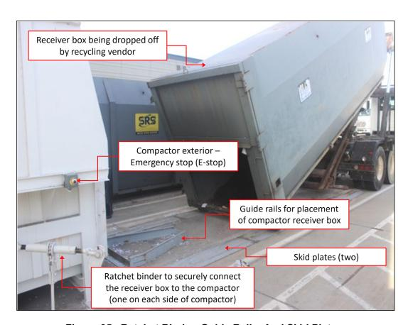
Figure 35. Ratchet Binder, Guide Rails, And Skid Plates
