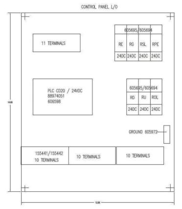
Figure 33. Operator Control Panel-Interior And Wiring Block Diagram
