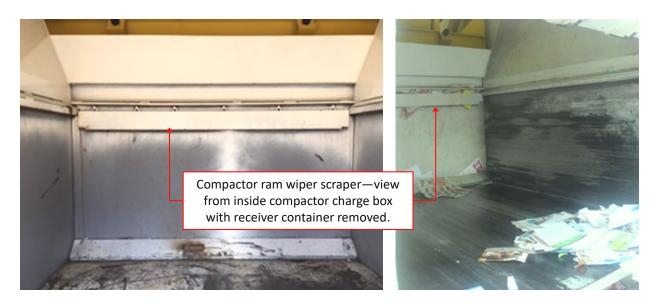
Figure 36. Compactor Ram Wiper Scraper
