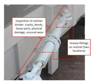
Figure 18. Grease Ratchet Binders
