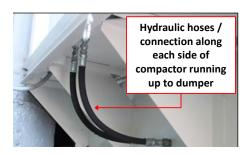
FIGURE 7. Check Hydraulic Hoses
