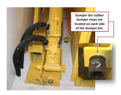
Figure 8. Rubber Bumper Stops
