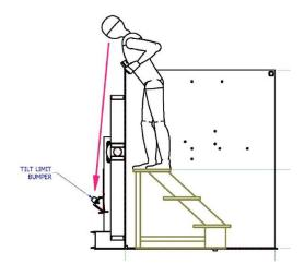
Figure 10. Checking Tilt Bumper
