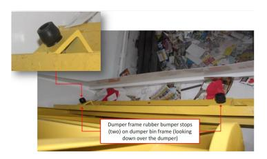
Figure 9. Frame Rubber Stops
