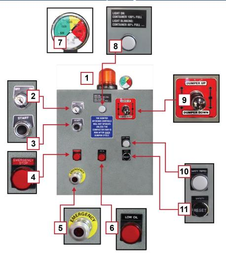
Figure 30. Operator Control Panel—Recycling Dumper/Compactor
