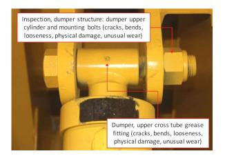
Figure 15. Upper Grease Fitting
