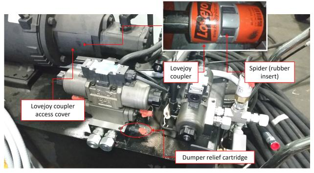
Figure 32. Hydraulic Power Unit—Detail Components
